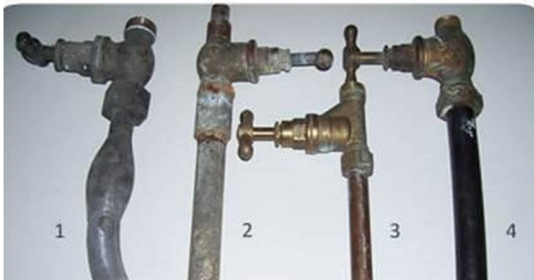
1. Lead 2. Steel 3. Copper 4. Plastic
